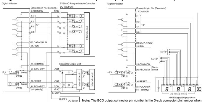
the BCD Output Cable (sold separately) is connected. This number differs from the pin number for the Digital Indicator narrow pitch connector (manufactured by Honda Tsushin Kogyo Co., Ltd.).
