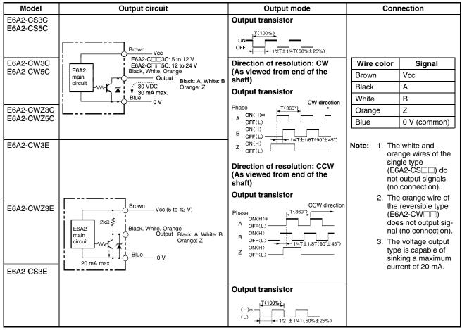
Note: 1. \*(H) and (L) indicate the output levels of the voltage output type.
