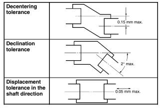
If there is a difference in angle or position between the shaft and the other shaft connected, an excessive load that may damage the shaft will be imposed on the shaft. Make sure that the shaft is connected properly.
