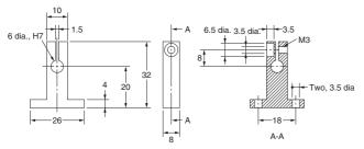
Mount the Sensor Head using M3 screws and a mounting torque between 0.6 and 0.8  $\mbox{N} {\cdot} \mbox{m}.$
