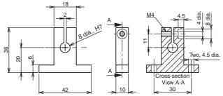
Mount the Sensor Head using M4 screws and a mounting torque between 2 and 3  $\ensuremath{\text{N}}\xspace\text{-}\xspace\text{-}\xspace$  mounting torque between 2 and 3  $\ensuremath{\text{N}}\xspace\text{-}\xspace\text{-}\xspace$  mounting torque between 2 and 3  $\ensuremath{\text{N}}\xspace\text{-}\xspace$  mounting torque between 2 and 3  $\ensuremath{\text{N}}\xspace$  mounting torque between 2 and 3  $\ensuremath{\text{N}}\xspace$
